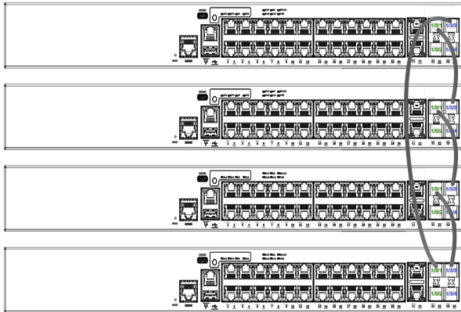
FIGURE 9 ICX 7150 24-port Stack Ring Topology
