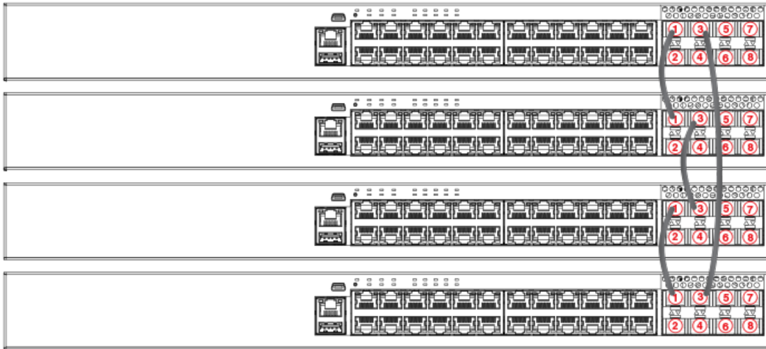
FIGURE 15 ICX 7250-24P Ring Stack
