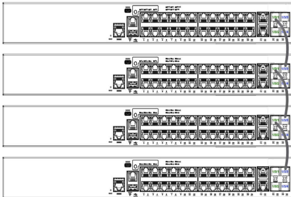
FIGURE 8 ICX 7150 24-port Model, Linear Stack
