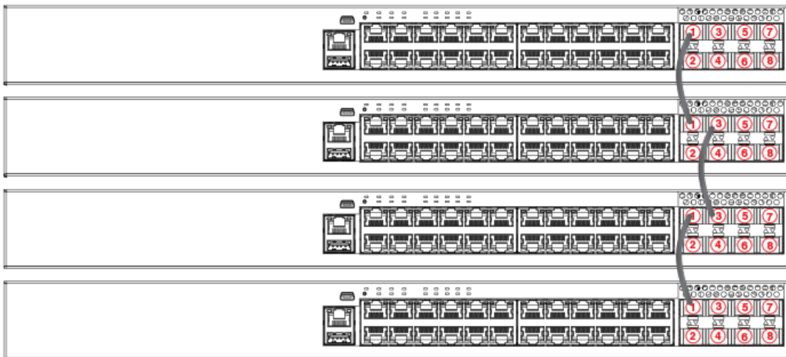
FIGURE 14 ICX 7250-24P Linear Stack
